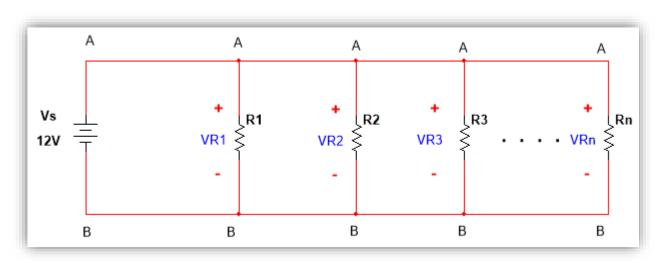
$$V_{AB} = V_S = V_{R1} = V_{R2} = V_{R3} = \dots V_{Rn}$$
