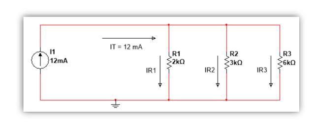
•  $I_{R3} = I_T \times \frac{R_T}{R_3} = 12 \times \frac{1K\Omega}{6K\Omega} = 2 \text{ mA}.$
