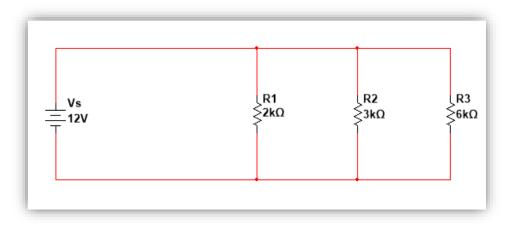
$$I_{R3} = \frac{V_{R3}}{R3} = \frac{12 V}{6K} = 2 \text{ mA}$$
